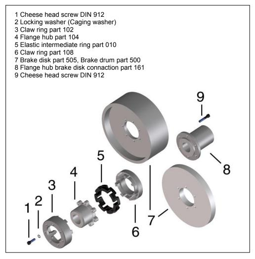
Fig. 1 Construction RINGFEDER® TNM GHBS
